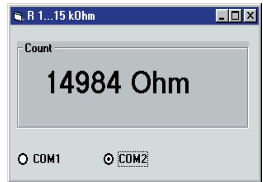
Figure 11. Measurement using a 15 \text{ k}\Omega resistor.
